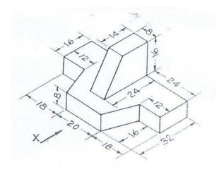
**8.** Draw three views of the blocks shown pictorially in figure according to [10M] first angle projection
