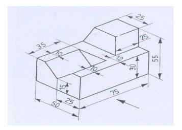
**8.** Draw three views of the blocks shown pictorially in figure according to [10M] first angle projection
